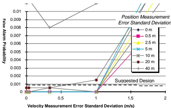
**Figure 3. 2,500 ft Independent Runway False Alarm Scenario: Sensitivity to Position, Velocity Errors**
