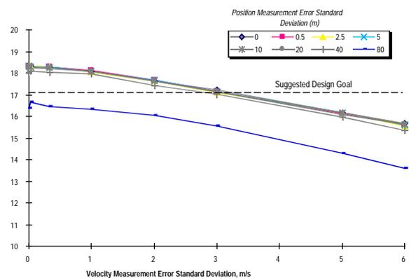
**Figure 1. 2,500 ft Independent Parallel Runway: Sensitivity to Position, Velocity Errors**
