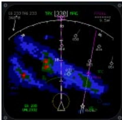
**Figure 5. TCAS Navigation Display with Overlay of CDTI Enhancements**
