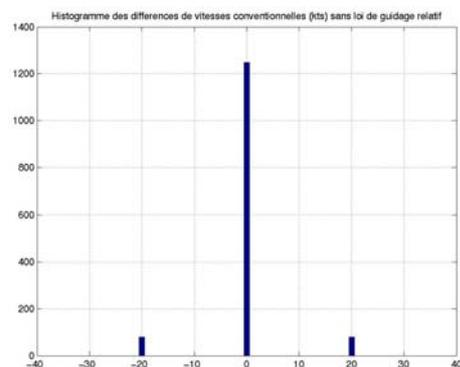
**Figure 7. Difference between the conventional airspeed of the two aircraft at the sequencing measurement point without any feedback loop**
