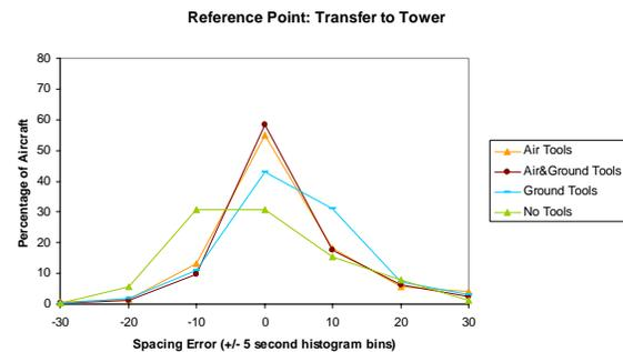
Figure 5. Spacing accuracy histogram measured upon transfer of communication to Ghost Tower.
