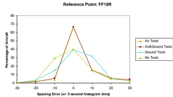
Figure 4. Spacing accuracy histogram measured at the Final Approach Fix for runway 18R.
