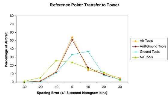
**Figure 8. Spacing accuracy for aircraft in uncoordinated flows.**
