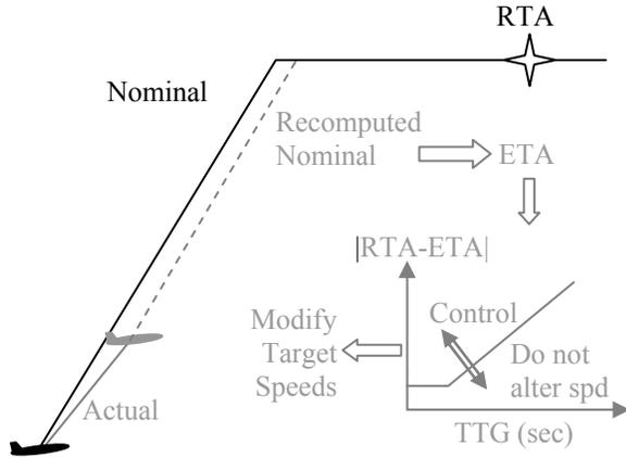
**Figure 2 Illustration of RTA Algorithm**
